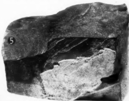
Fig. 5—Example of cement (1/32 in. thick) which set up in fracture in Spraberry.
